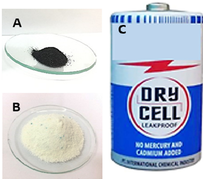
Fig. 1. The materials used in this study are (A) graphite powder from the battery waste, (B) commercial detergent, and (C) a ZnC battery.
